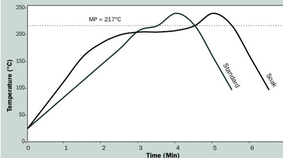
The stated profile recommendations apply to most Pb-Free alloys in the Sn/Ag/Cu (SAC) alloy system, including SAC 305 (96.5Sn/3.0Ag/0.5Cu). This can be used as a general guideline in establishing a reflow profile when using **Indium8.9** Solder Paste. Deviations from these recommendations are acceptable, and may be necessary, based on specific process requirements, including board size, thickness & density.
